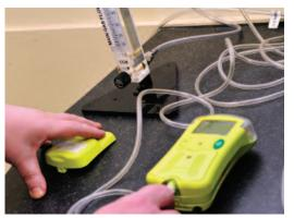
RCS will calibrate the flow meters on air samplers and air monitors against a flow rate standard, which is traceable to national standards. In addition RCS own a range of test sources which are suitable to calibrate the radiation detector in air monitors. All testing is undertaken in accordance with GPG No.82.
