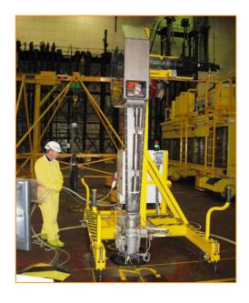
The condition of the fuel elements, held in the site's 'dry storage cells' meant they could not be safely removed by the standard fuelling machine grab. JFN undertook the design, manufacture and testing of a bespoke fuel retrieval system - incorporating an electro-mechanical grab to remove the fuel elements.
