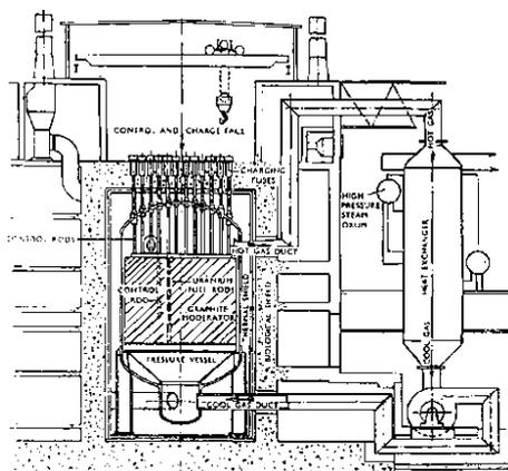
FIG. 1 Schematic of Calder Hall, the first Magnox power station [1]
