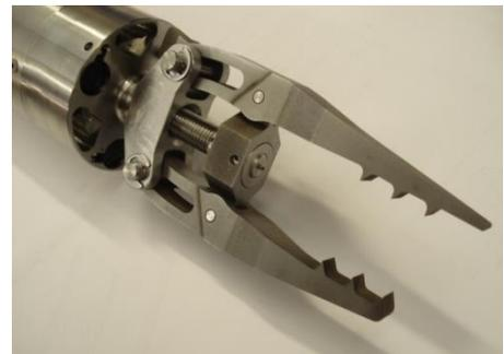
*FIG. 7 Completed grab mechanism*
