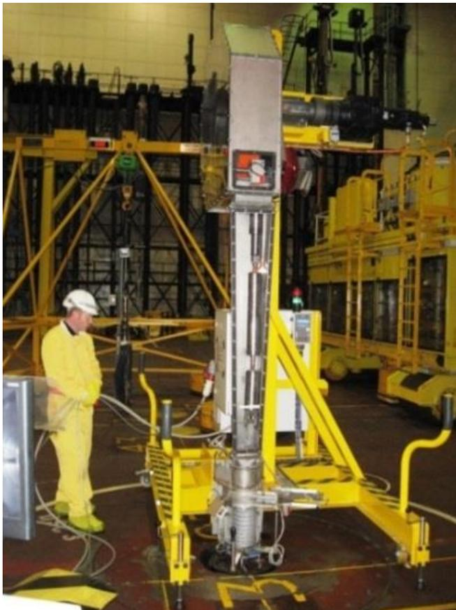
*FIG. 8 The finished machine in operation on the Pile Cap at Wylfa*
