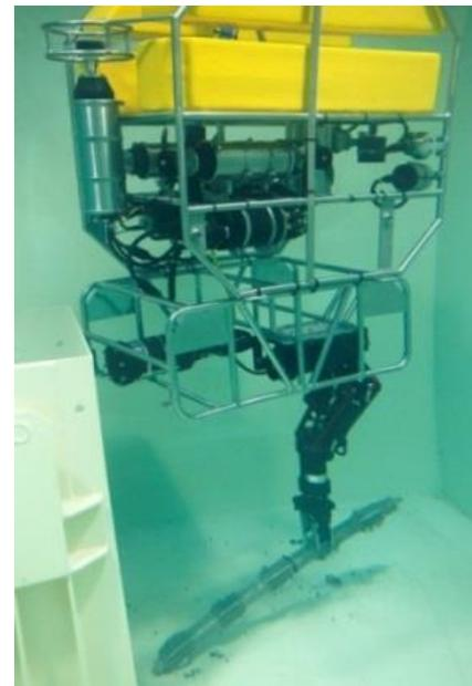
*FIG. 3 Hydraulic manipulator in use in the JFN test facility*
