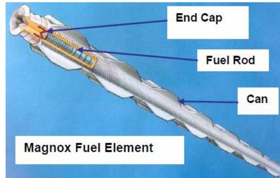
*FIG. 2 A typical Magnox fuel element with lifting button[2]*
