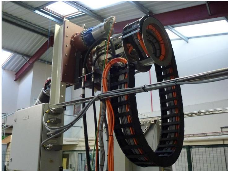
Figure 3 - Out-Cell Shoulder Drive & Valve Pack
