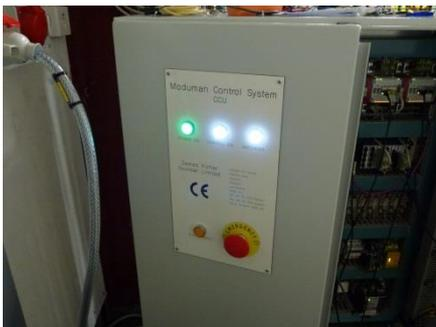
Figure 4 - Control Console Unit
