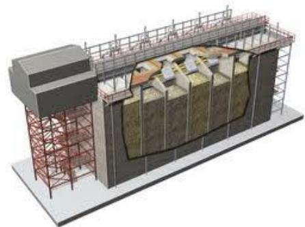
Fig 1 Pile Fuel Cladding Silo: photo of silo and cross section showing the silos
