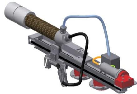
Fig. 10. Plate and Angle WJC Tool
