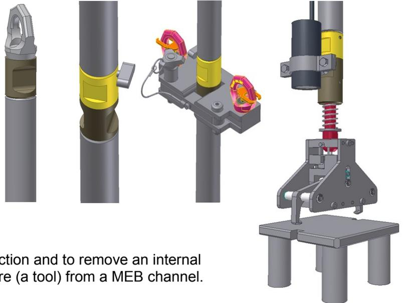
**JFN designed, manufactured and tested a long reach tool for the removal of a structural feature, known as a “stool” from a Multi Element Bottle (MEB)**
