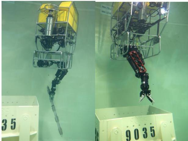
Hydraulic Manipulator deployed on the Seaker ROV
