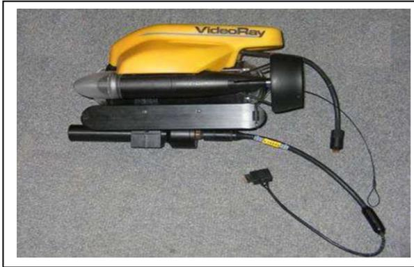
Gamma probe attached to the VideoRay Pro4
